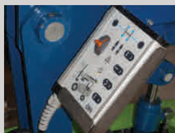
Wired remote control allows accurate placement of materials
