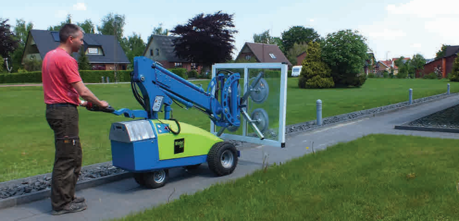
The Winlet 600 is narrow and its powered steering makes it highly manoeuvrable
