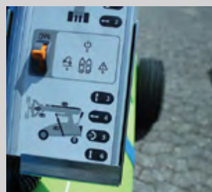
Multifunction control panel with integrated buttons and signal lights
